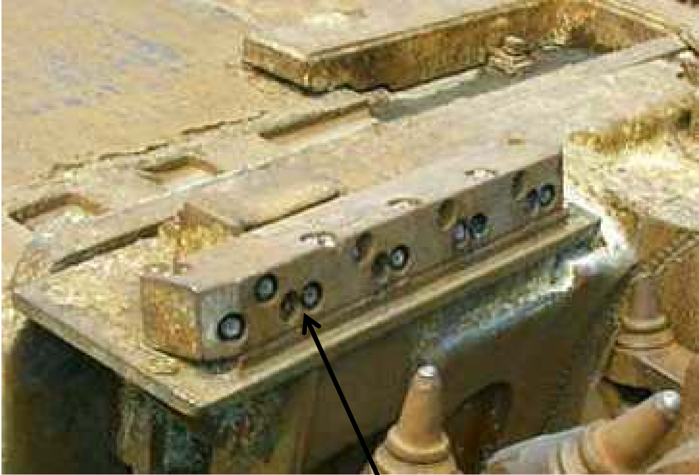
Multiple spray orientations with minimal spacing
