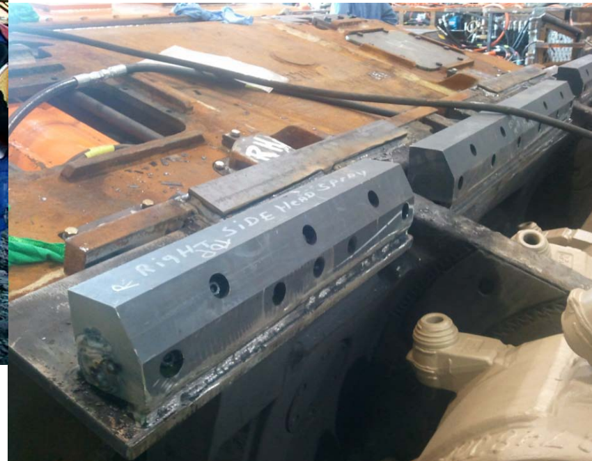
Installation of sprays at JOY rebuild center
